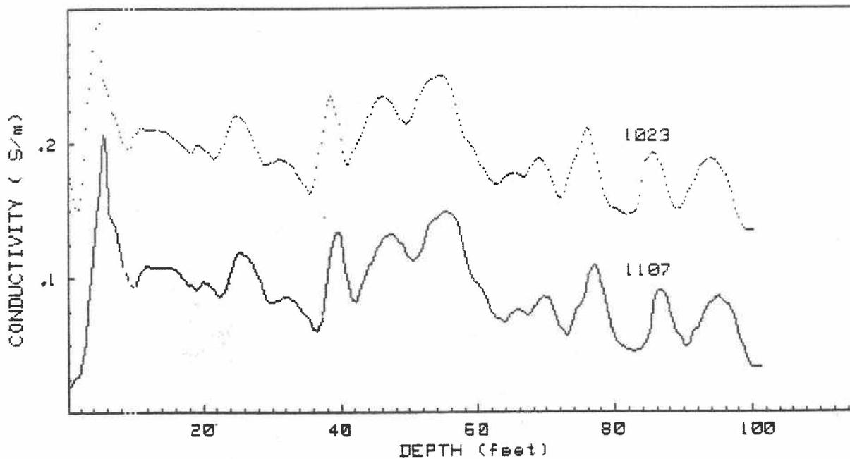
Figure 8. Data from observation well six, taken on October 23 and November 11, 1987. Data for October 23 is offset by 100 mS/m. Horizontal scale 1"=20', vertical scale 1"=100 mS/m.
