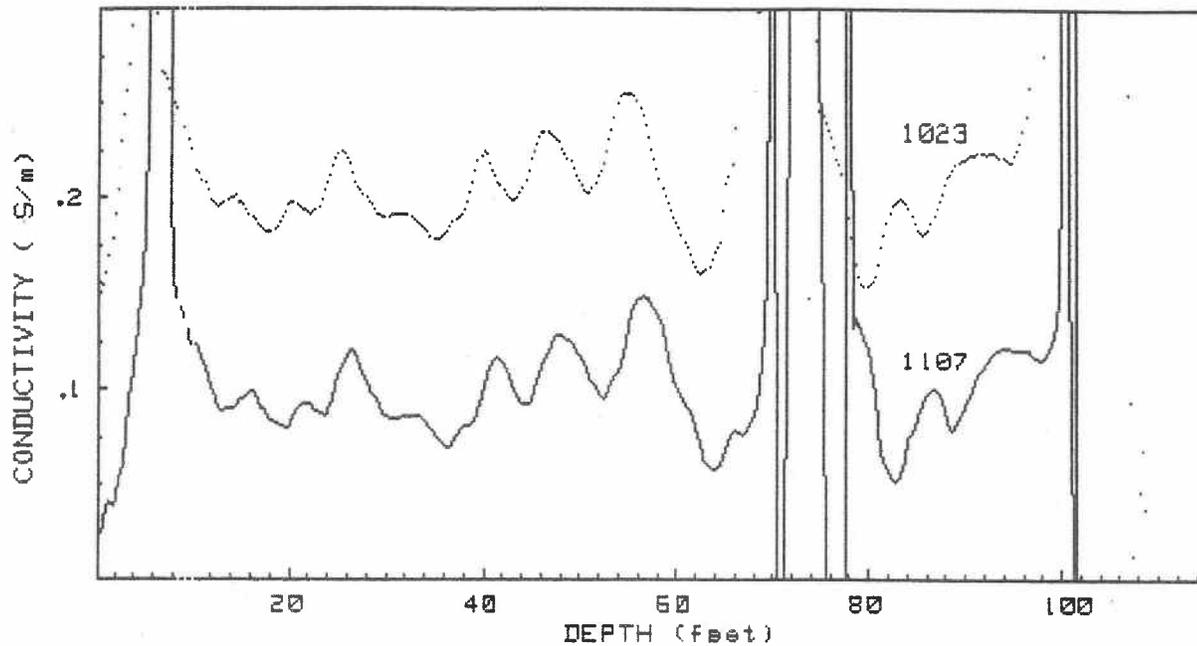
Figure 9. Data from the extraction well, taken on October 23 and November 11, 1987. Data for October 23 is offset by 100 mS/m. Horizontal scale 1"=20', vertical scale 1"=100 mS/m.
