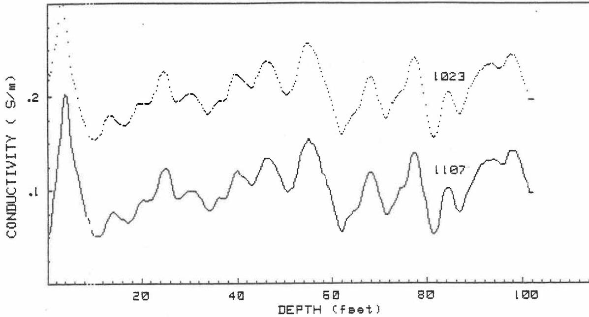
Figure 7. Data from observation well five, taken on October 23 and November 11, 1987. Data for October 23 is offset by 100 mS/m. Horizontal scale 1"=20', vertical scale 1"=100 mS/m.
