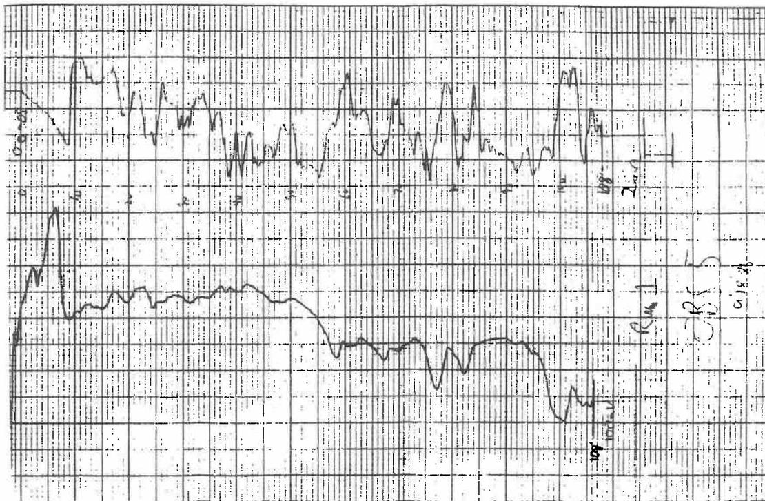
Figure 15. Resistivity and SP logs from observation well 5 taken on September 18, 1986.
