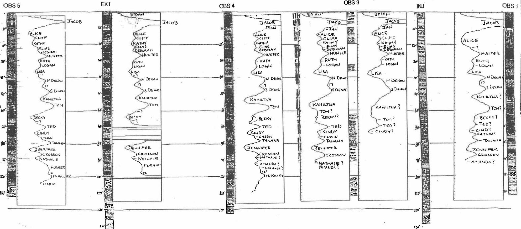
Figure 10. Electromagnetic induction logs along line AA', illustrating how names were assigned to anomalies.
