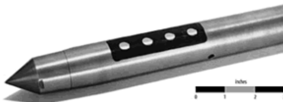
Electrical conductivity probe with Wenner array electrodes. Courtesy of Geoprobe Systems.
