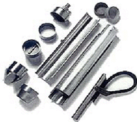
Split sampler with acetate liner
