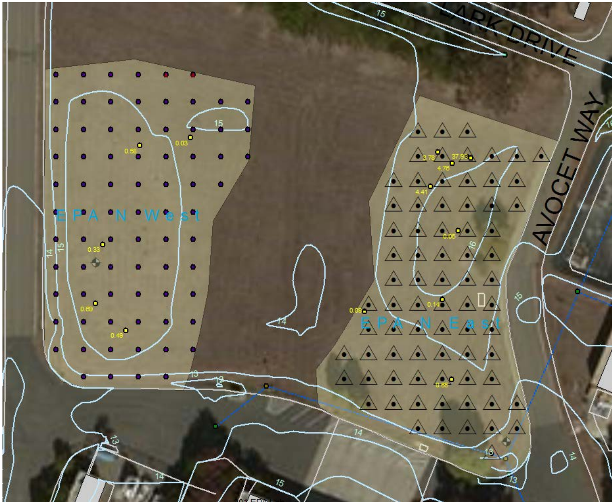
Figure 3. 75 increment grid for incremental sampling methodology increment locations.
