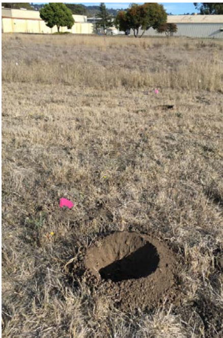
Example of an auger bit boring.
