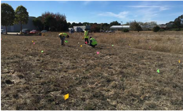
Placing ISM increment locations using the triplicate template
