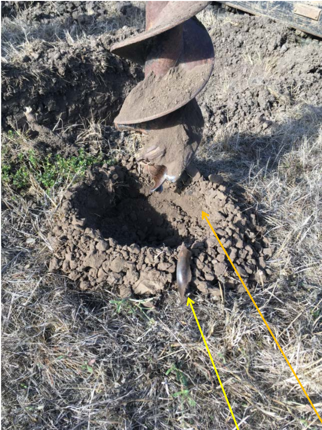
Example of distinction between native highly plastic silty clay prairie soils and gravelly fill material with auger tip showing above the hole. Samplers were instructed to avoid collecting native soils in increments if they did appear in the borings.
