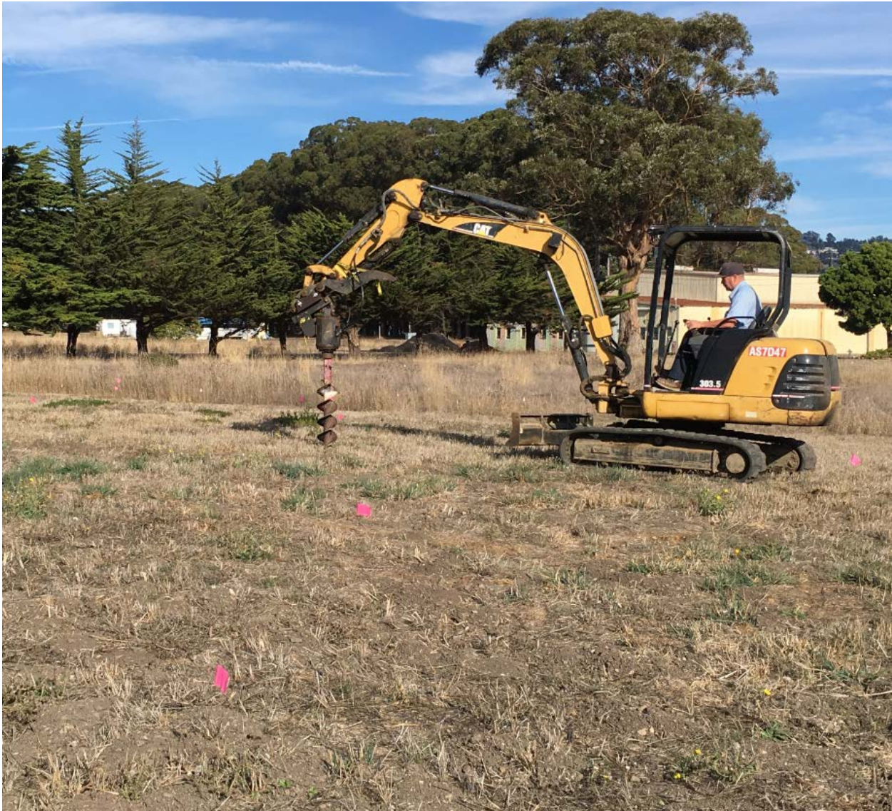
November 14, 2017 EPA Northeast pile decision unit showing use of auger bit.
