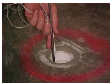
Initial insertion into permanent sampling port.
