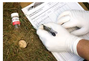
After insertion, impermeable cork sealed
