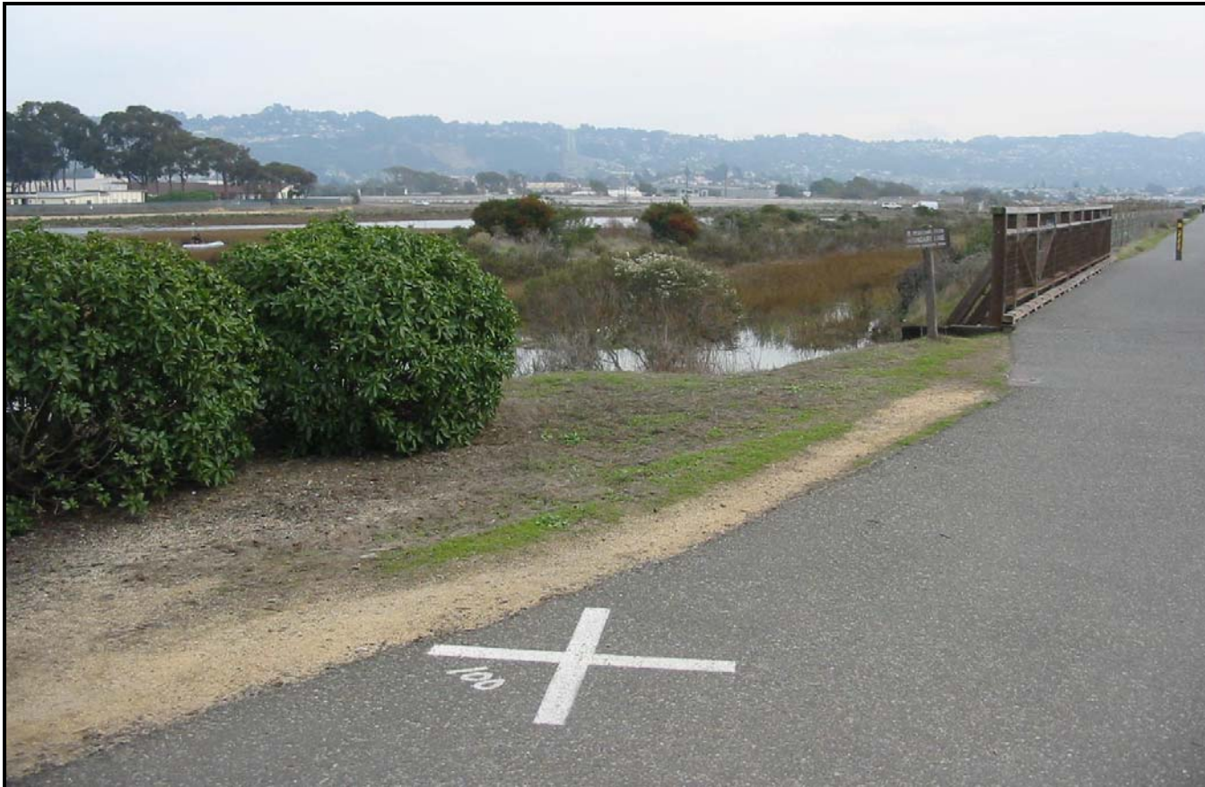
Figure A.12. Existing mark located on the EBRPD Bay Trail. The location was surveyed during the November, 2006 and August, 2007 surveys. No documentation of a previous survey of this mark is available for comparison. The marker is located at the southwestern corner of the study area. Photo dated 11/21/2006.
