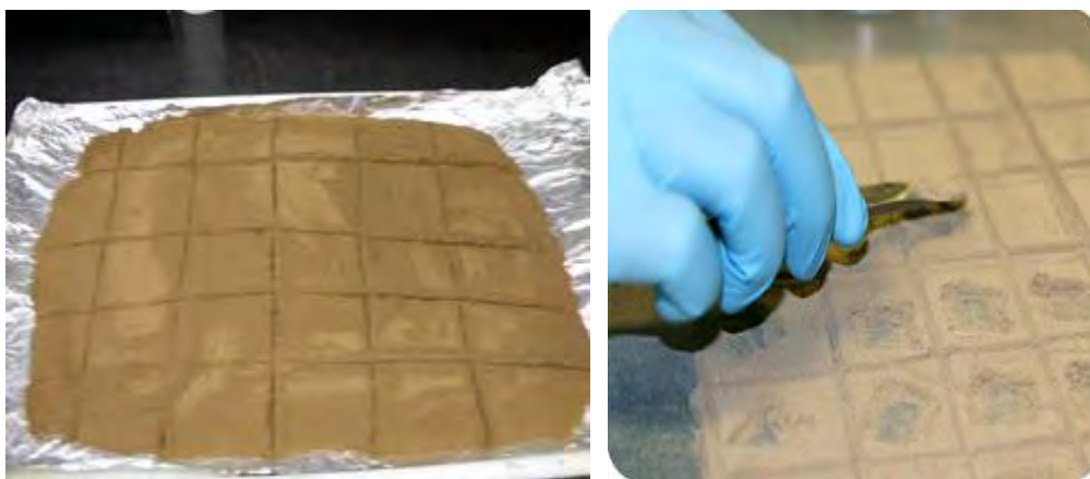
Figure 2 - 30 square grid marked on sample; sampling the grids
