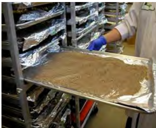
Figure 1 - Drying the (composited) sample
