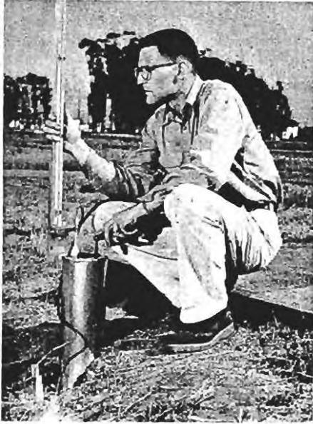
FIGURE 5a. Sampling well head and mercury pot manometer
